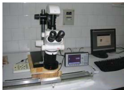
Stereo-zoom microscope with TA system for tree ring analysis
