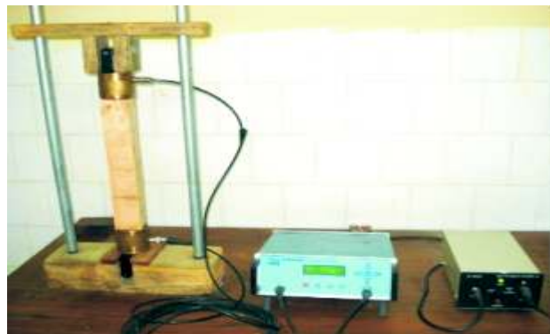
Ultrasonic Technique on Standing Trees for Defect Detection
