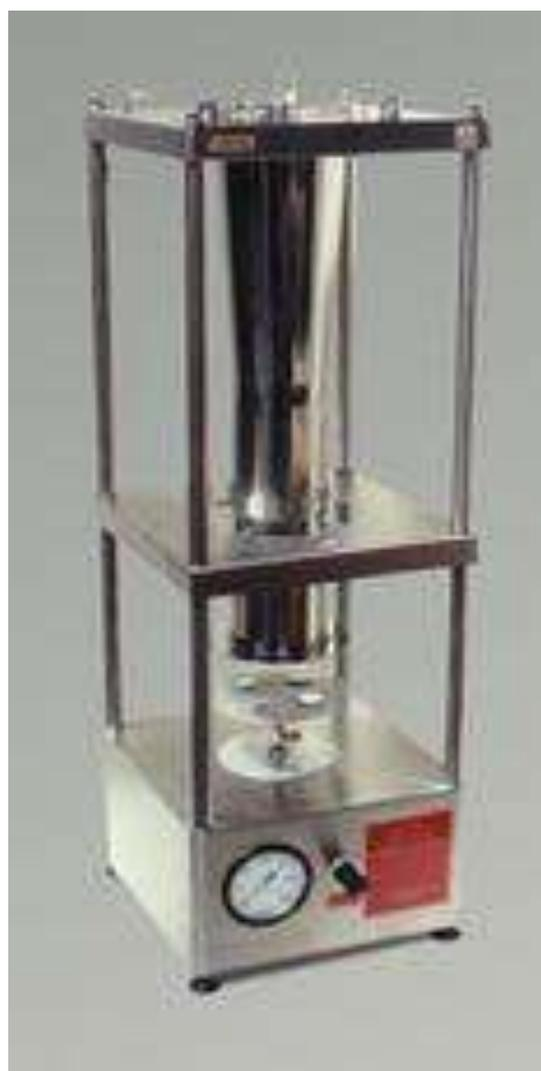
pneumatic on/off switch mounted outside
