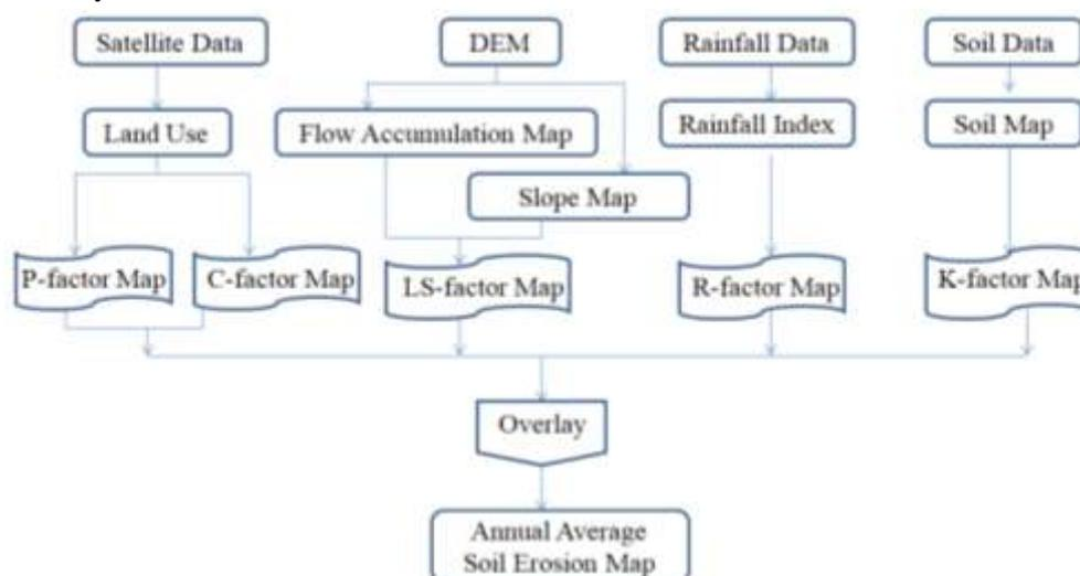
**Fig 1: Flow chart for estimation of annual rate of soil erosion using RUSLE and Remote sensing and GIS**
