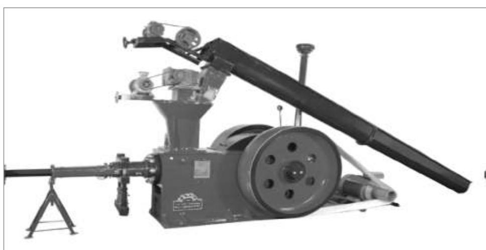
Fig 1. Biomass Briquetting Machine
