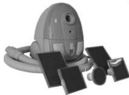
It is used for seed counting and also placing the seed in petridish or germination tray in the course of seed germination. It has a suction tube and suction head with control button to control the suction power according to seed size.
