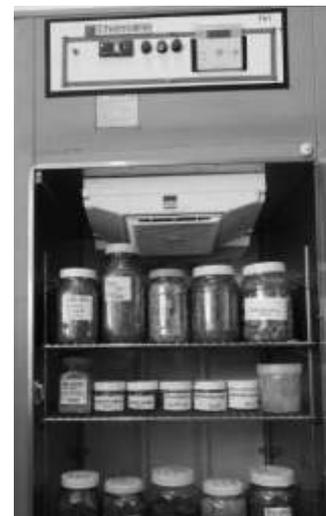
The Seed Storage Chambers are basically enclosed spaces with a controlled environment, designed to maintain specific temperature and relative humidity conditions for short term or long term storage of seeds. Seeds with reduced moisture content (desiccated) are stored at desired low temperature for enhancing the shelf life.
