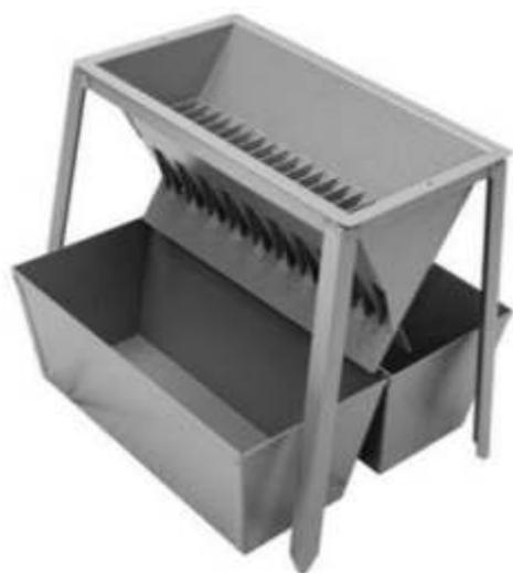
It is precisely designed to reduce the bulk of material to a convenient representative size for laboratory analysis. A homogenous, dry, free-flowing sample is poured evenly into the hopper/funnel. The material flows through the alternately arranged passages in the opposite direction (chutes/riffle bank) into the two collecting pans under the dividing head outlets. With
