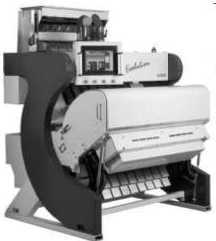
The colour separator is used to separate discoloured seed, greatly of lower quality. Separation based on colour is necessary because the density and dimensions of discoloured seed are the same as those of sound seed; Seed that differs in colour is detected by the photo cells, which generate an electric impulse. The impulse activates an air jet to blow away the discoloured seed into reject bin while the rest of the seed passes through to another bin.
