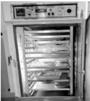
It is basically a growth chamber that creates an artificial environment of temperature, humidity and light to provide optimum conditions for the germination of seeds. Temperature of the chamber can be altered to constant high or low temperature for different time periods. The germination chamber, improves uniformity, decreases the lead time and increases the numbers of germinating seeds.
