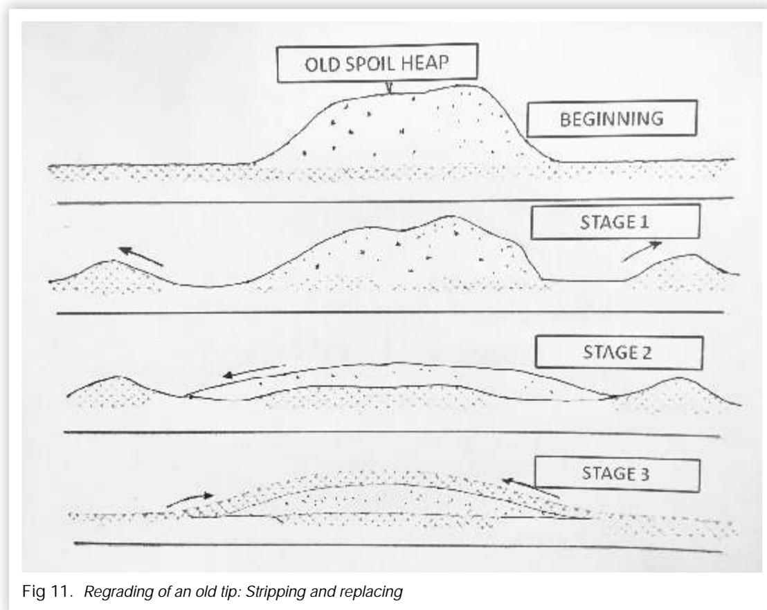
Fig 11. Regrading of an old tip: Stripping and replacing
