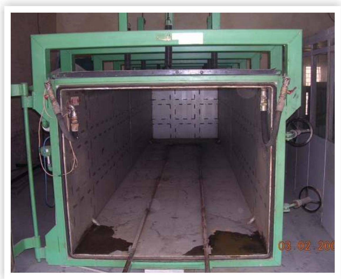
Conduction heating based vacuum kiln at FRI
