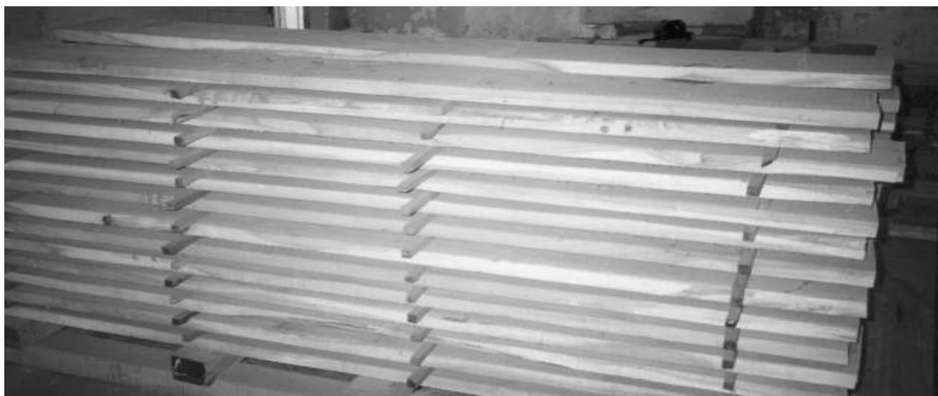
Stacking of timber using spacers
