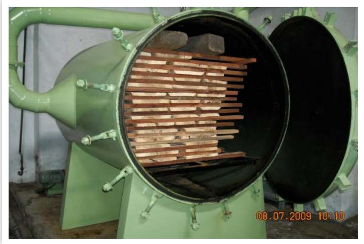
FRI Convection heating based Vacuum Kiln
