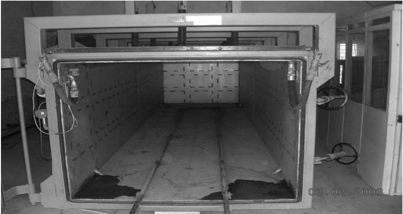
Hot press (conduction heating) type Vacuum kiln at FRI
