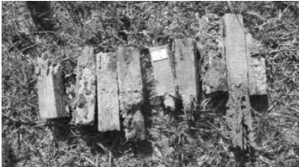
Natural Durability test of imported timber in field
