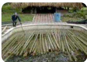
Soaking bamboo culms in water to leach out starch
