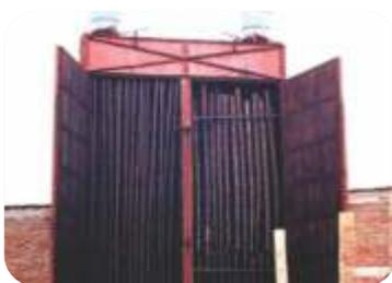
Culms stacked in a heating chamber
