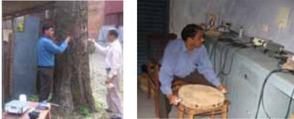
**Defect detection in timber by ultrasound**
