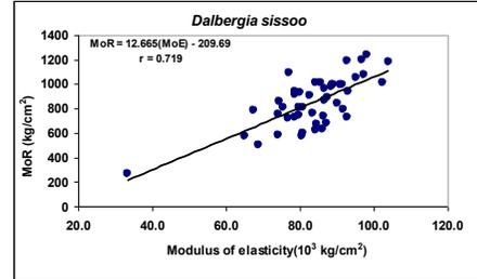
Fig.- 3. Modulus of rupture as a function of modulus of elasticity.
