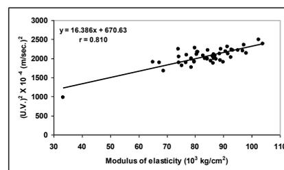
Fig.- 1. Square of ultrasonic velocity as a function of modulus of elasticity
