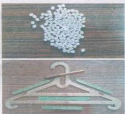
Clockwise from top: Dr Pankaj Aggarwal (in white shirt) and Dr S S Chauhan working at the extrusion system. Polymer granules extracted from polylactic acid. Pen, hanger and sticks made of wood plastic
