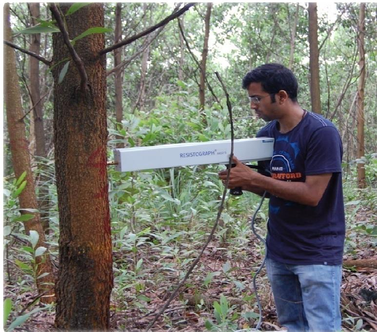
**Shri Uthappa, trainee measuring wood density using resistograph**
