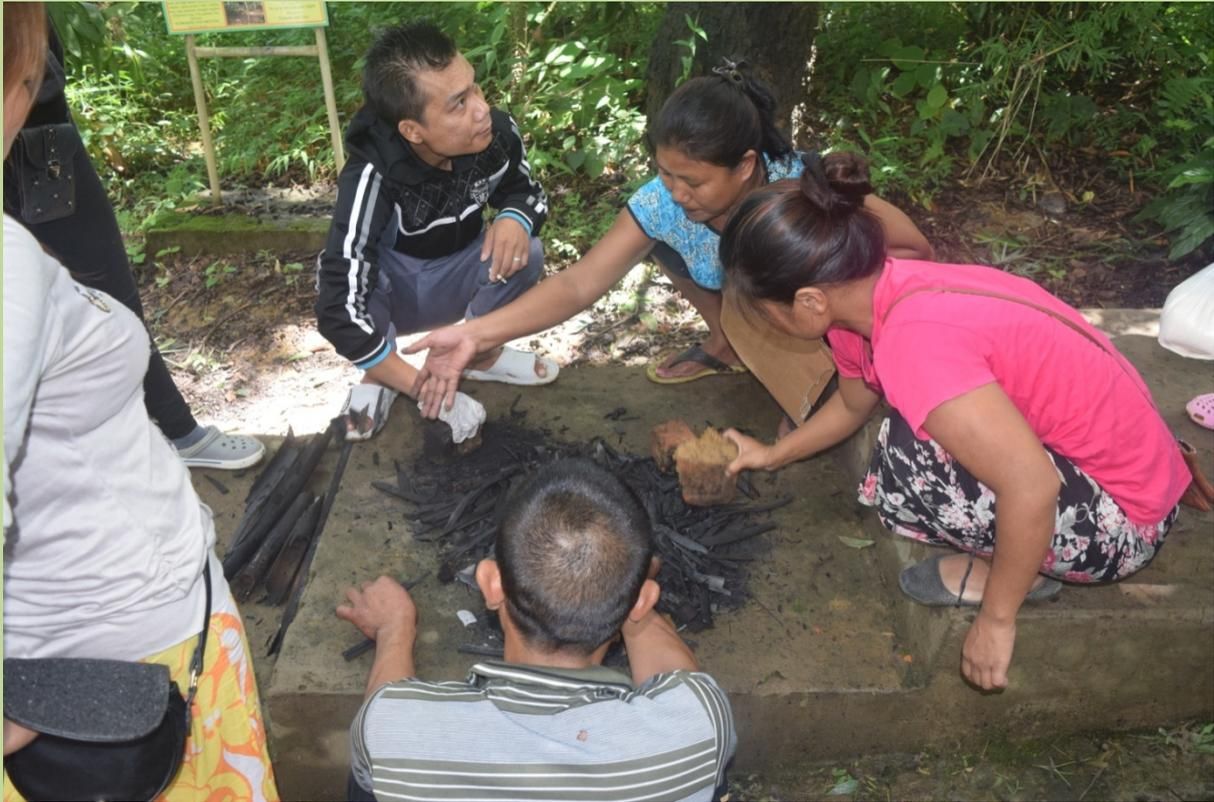
**Figure 13: Raw Bamboo Charcoal is crushed to make bamboo charcoal briquettes.**
