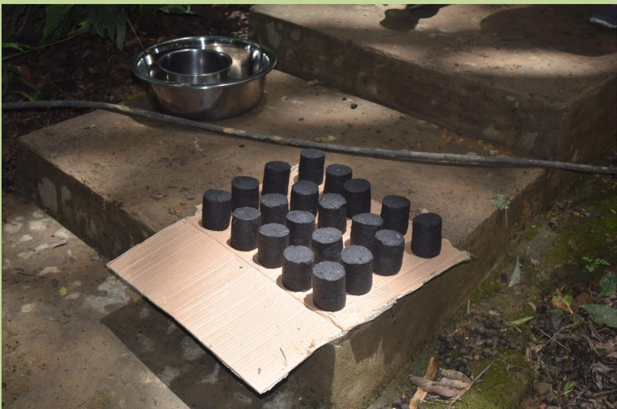
**Figure 16: Bamboo Charcoal briquettes are placed under sunlight for drying.**
