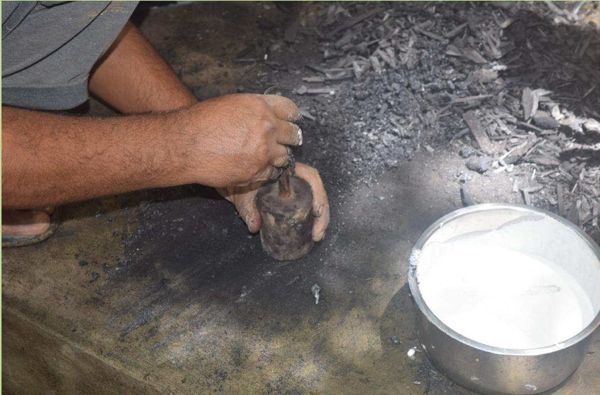
**Figure 15: Mixture of powdered bamboo charcoal and binder is compressed through moulds to make briquettes.**
