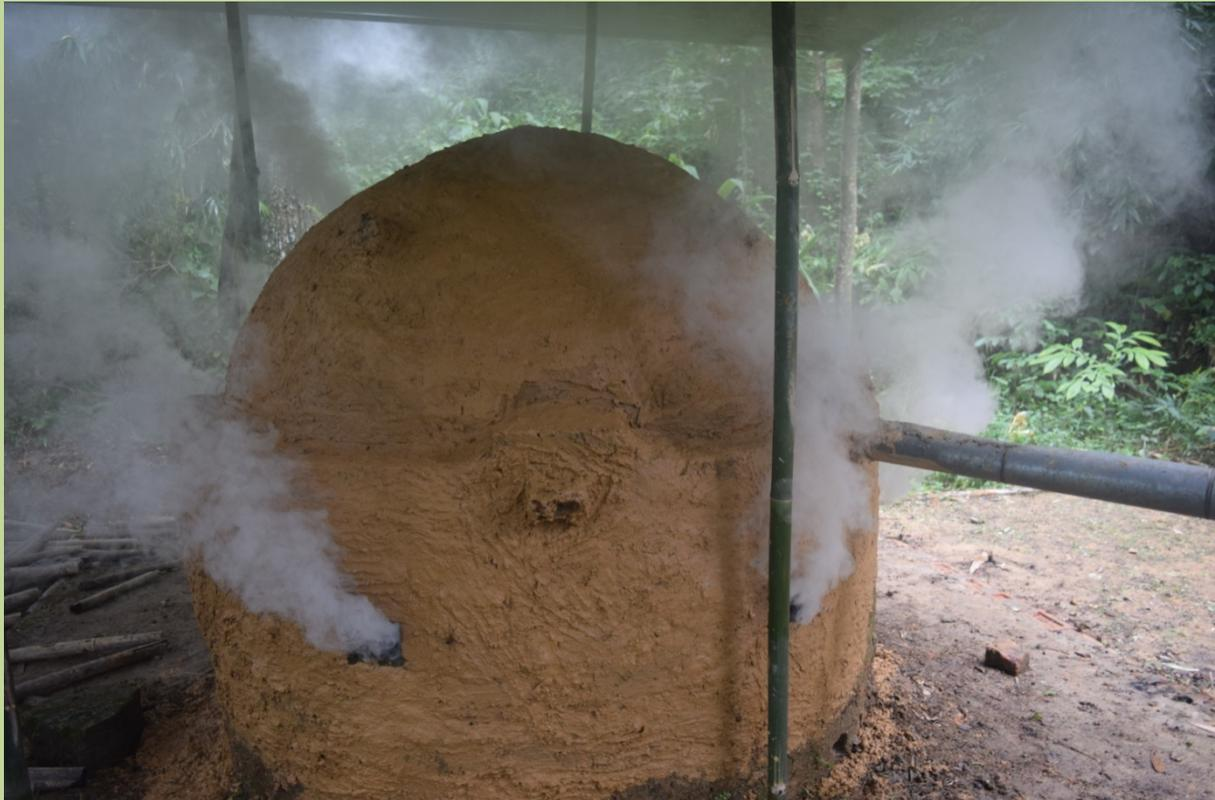
**Figure 11: Bamboo Charcoal Kiln in operation during training.**
