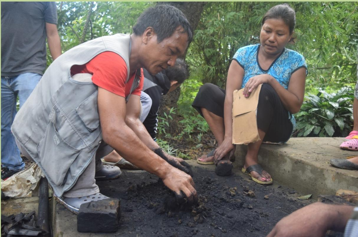
**Figure 14: Powered Bamboo Charcoal is mixed with suitable binder to make briquettes.**
