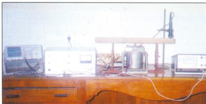
Method to measure the strength properties (MOE) of wood using sonic waves.
